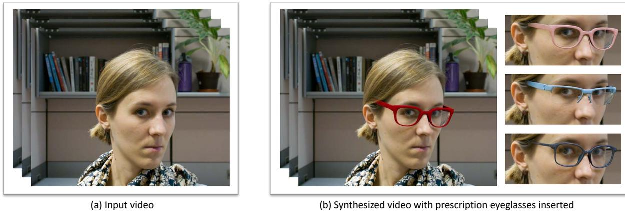
Fig. 2. Our virtual try-on system for prescription eyeglasses modifies an input video (a) and virtually inserts prescription eyeglasses, producing an output (b) similar to a virtual mirror. Our approach handles reflection and shadows, and simulates the effects of refraction according to the user’s eyeglasses prescription. A variety of eyeglasses frames are available for selection.
