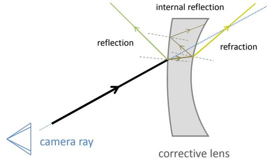
Fig. 4. Illustration of ray tracing for simulation of the refraction and reflection effects. As camera rays (blue) enter the first surface of a corrective lens, each ray is refracted or reflected, either into the lens or back into the scene. For some of the rays entering the lens, total internal reflection occurs.
