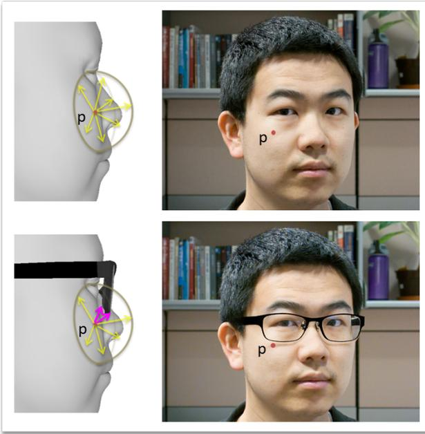
Fig. 5. Illustration of the Monte Carlo integration process, for shading computation. In order to estimate the shading at a point  $\mathbf{p}$ , rays are traced from  $\mathbf{p}$  to several directions of the viewing hemisphere (top). Once virtual eyeglasses are inserted (bottom), the eyeglasses frame blocks some of these rays (rays in magenta). This results in shadows cast on the user’s face, which our approach is able to simulate.
